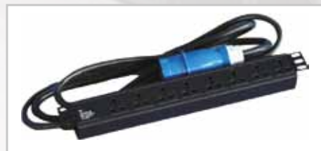
8-outlet All usage PDU, 2P+E industrial plug 32A input 10A all usage outlet, without switch, 3.0m length cable, 19" positive installation with Smartnet logo (322000796)
