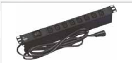
8-outlet PDU, IEC320 C14 plug 10A input, EC320 C13 outlet 10A output, with master switch, 3.0m length cable, 19" positive installation with Smartnet logo (322000742)
